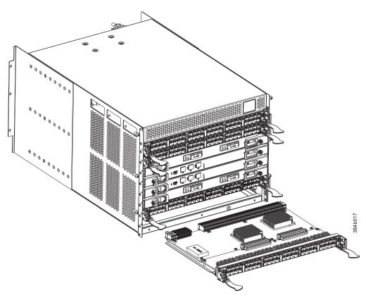
Figure 33. Port blade removal and installation (48-port blade shown as example)
